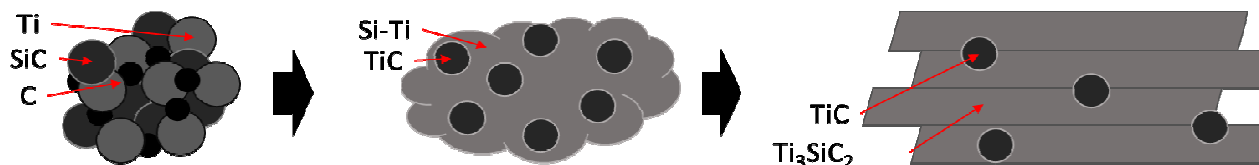
Fig. 2. Scheme of MAX phase formation in Ti-Si-C system
