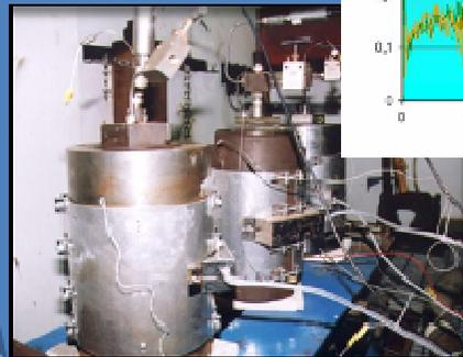
Pressure vessels for H<sub>2</sub>S exposure
