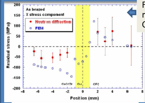
FEM calculation for the residual stress in a C/C-Cu joint
