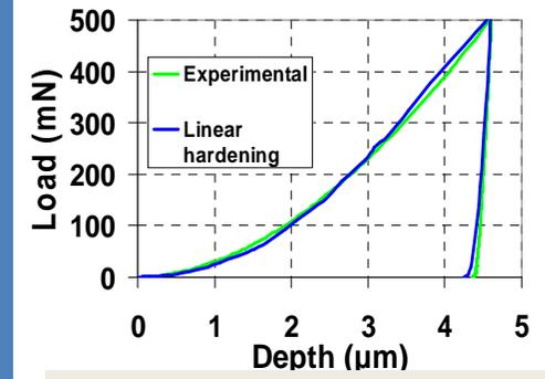
load vs penetration-depth curves while indenting the stressed metal phase (Cu)
